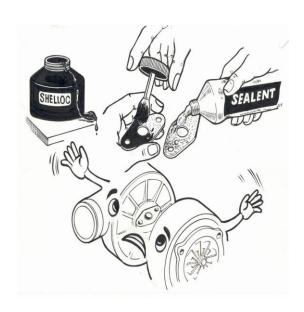
Do not apply gasket sealant pastes at oil inlet flange
