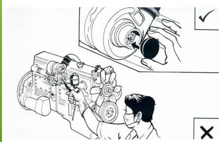
Close the TC openings with proper protective plugs before cleaning the engine.
